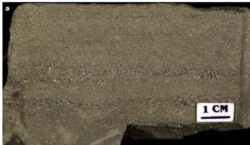
Figure A2.1a. Baker Patton Cu deposit, surface trench sample. Very oxidized, pyrite-rich massive sulphide. Sample 06AV-501.
