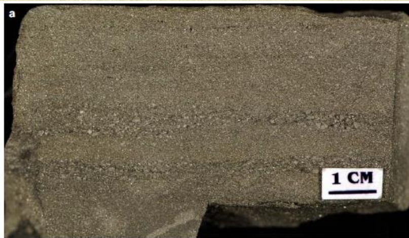
Figure A2.1a. Baker Patton Cu deposit, surface trench sample. Very oxidized, pyrite-rich massive sulphide. Sample 06AV-501.
